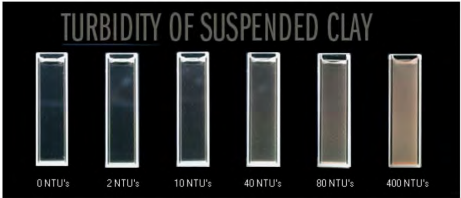
Plate 1. Visual NTU scale for assessing Turbidty. ©WOW (1999 - 2004).
